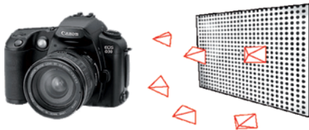
A typical digital camera with calibration target and camera positions tagged by pyramids
